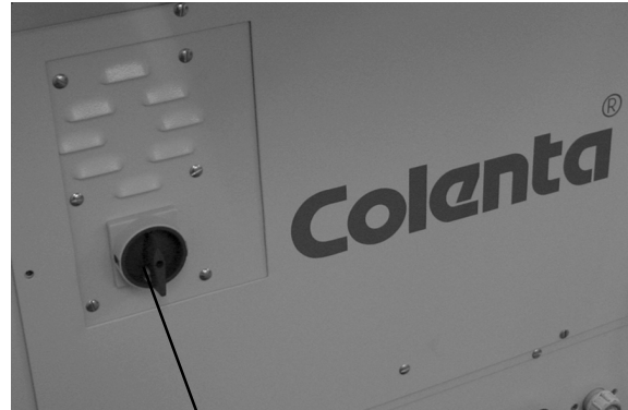
Main switch For the FEEDER and the FILMPROCESSOR!
