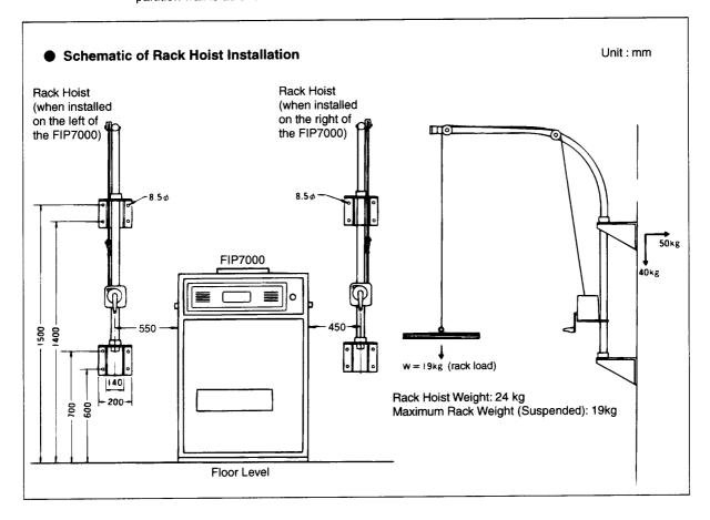
3. Use M8 bolts to fasten the rack hoist to the partition wall.
