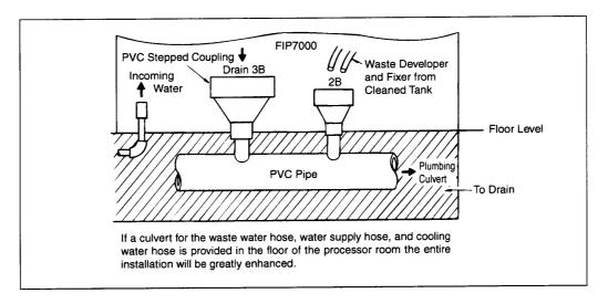
Since the drain opening is not closed up, provision should be made for trapping sewer gas and odors.
