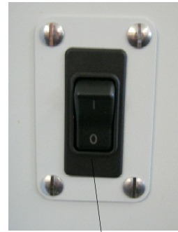
Main power switch
