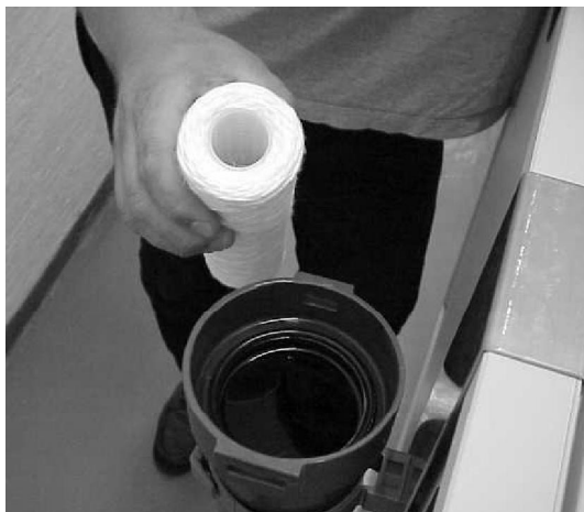
7. close the filter system in the reversed sequence as described before (step 2)
