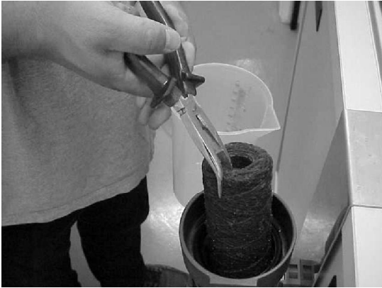
5. check position of the O-ring inside filterhousing
