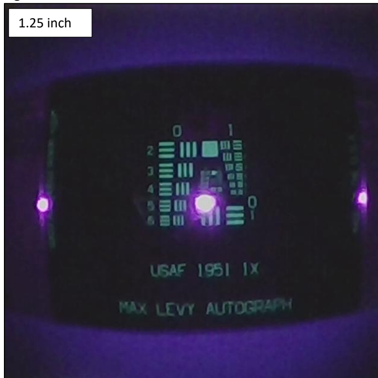
Fig 8. USAF 1951Resolution Chart at 1.25"
