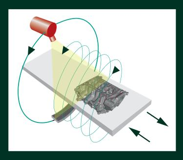
With the high-speed automatic helix CT, a gantry with a X-ray tube and corresponding 64 channel multi-line detector rotates around the work piece being forwarded on the manipulation table.
