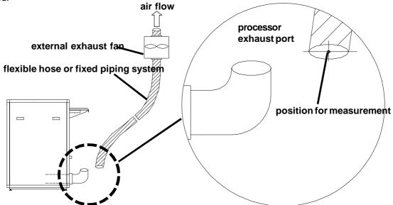
NOTE: If the ventilation tubing is connectet to house-internal exhaust system, an air-gab of 5cm (2 inch) has to be provided accordingly.
